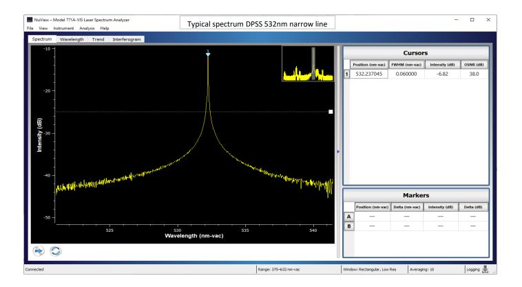
The Lambda-Beam is a narrow linewidth 532nm DPSS green laser which delivers up to 200 mW of low noise output power. These modules are designed for demanding applications that require both high stability and excellent beam quality. They offer user adjustable output power, a USB interface (RS232 optional) and control software.
