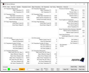
The included TEC Service Software is a powerful tool that allows monitoring, data logging and full configuration of the TEC-1091 via a standard USB or an RS485 / RS232 TTL connection from a PC running Windows.
