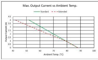
Standard or Extended Device Temperature Mode can be set as software setting. Using forced air cooling, it is possible to enhance the ambient temperature performance.
