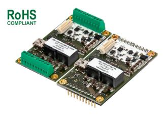
The TEC-1091 is a specialized TEC Controller / power supply able to precision-drive a single Peltier element.
