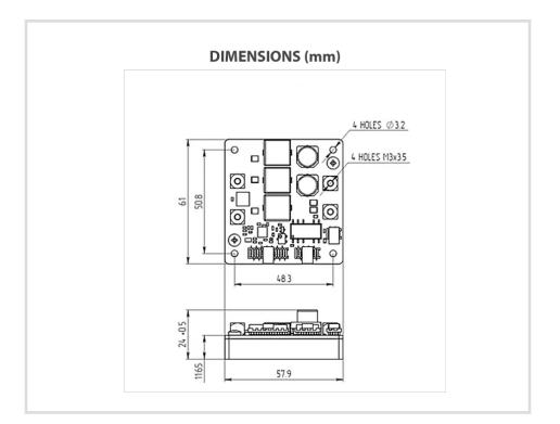
Product includes control software GUI for simple set-up and monitoring of your laser diode; alternately - you can use the trim pots on the board or the analog control connector
