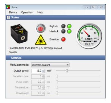
To install the software, simply run the setup file from the CD-ROM included in the package. The setup package then installs the application software and the device driver. For the operating system to properly recognize the device, it's best if you install the software first before attaching the device.
