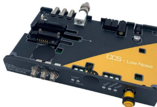
Multiple layers of laser diode protection ensure that your device is protected at all times. The drivers can be delivered with or without butterfly mounting sockets. They are compatible with butterfly laser diodes and many other form-factors (TO, TOSA, VCSEL etc.)
