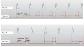
Exemple of two simple using cases: Digital delay (top) and frequency divider (bottom)
