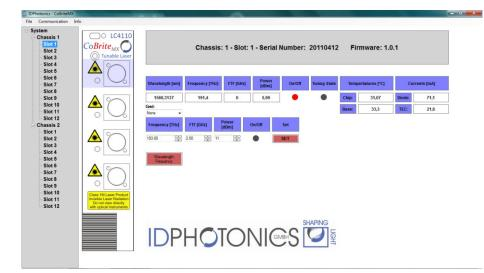
Click on any port to access parameters of laser ports located on that card which are represented in the left hand side of the GUI. Refer to section 5.5 on features available by this table.
