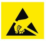
This sign indicates that the respective modules, boards or RF inputs and outputs are susceptible to damage by electro static discharge (ESD), and require proper protection procedures for storage and handling.
