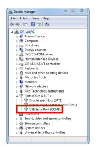
If no matching COM Port can be identified or an "unknown device" is displayed, the driver is not installed correctly.
