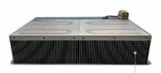
High fin density heat sink is enclosed in a sheet metal duct to direct the entire volume of forced air over the fins - this design helps provide a low thermal resistance of 0.04 °C/W
