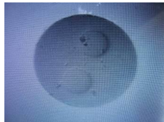
Dirty: Cleaning required
