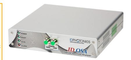
ID OSA is a versatile Optical Spectrum Analyzer for R&D and production test applications with picometer class spectral resolution across the C Band. It makes it a cost effective solution for spectral monitoring.
