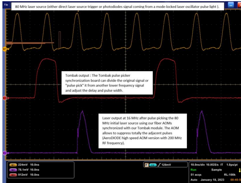
Figure 8 Pulse-picking measurement result.
