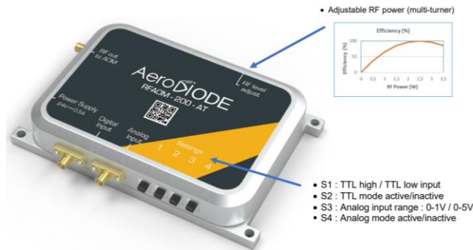
Figure 2 : Model RFAOM-TA-200 S1-S4 settings
