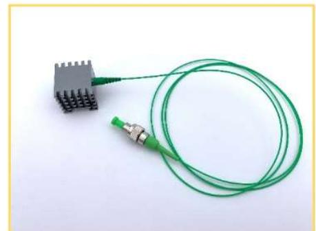
14 pin DIL supplied with a butterfly laser diode driver adaptation kit.
