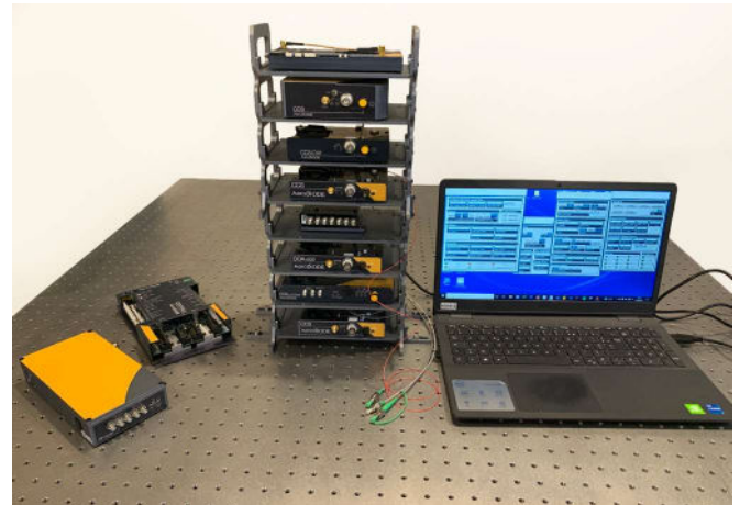
➤ All AeroDIODE products can be connected together (daisy chain) to a unique GUI interface which consolidates all modules functions
